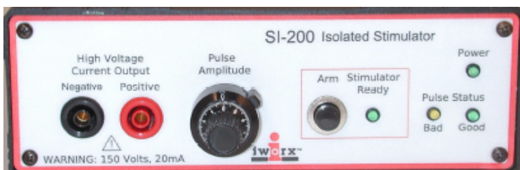
Figure 8A. The SI-200 isolated stimulator, front panel.
