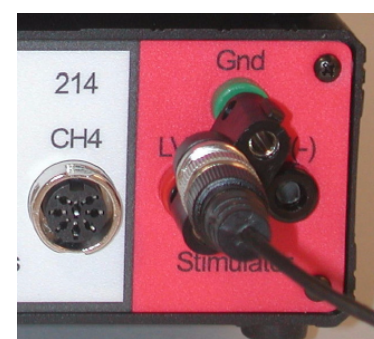
Figure 10. BNC-banana adapter connected to the iWorx 214 unit.
