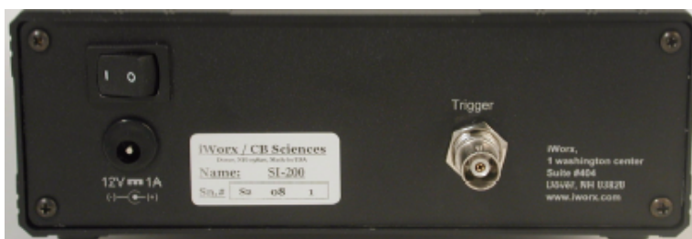
Figure 8B. The SI-200 isolated stimulator, back panel.
